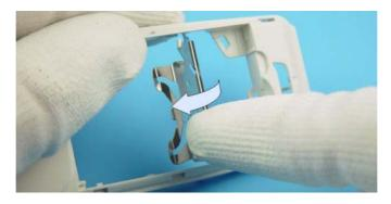
20. Expand the B-cover carefully and remove the SIM flap.
