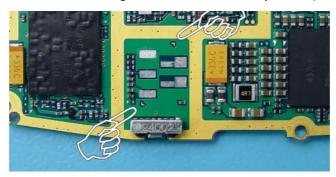
4. Tin one of the pads to fix the connector before soldering the following pins.
