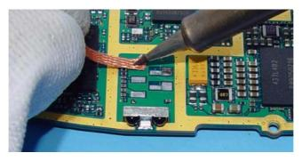
Note the location markings to fit the connector precisely.
