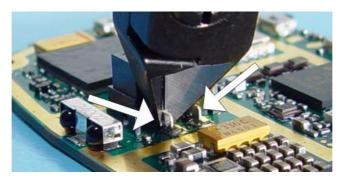
2. Push tweezers into the outside openings of the battery connector and lift up the plastic cover.
