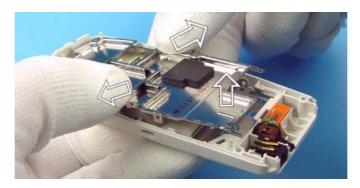
11. Remove the power button key.
