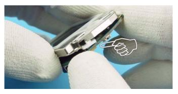
6. Separate the UI shield from the system module carefully. The key dome is attached with adhesive tape, which must not be touched.
