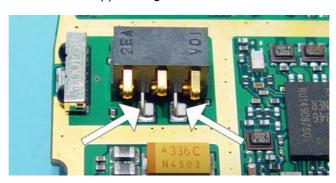
1. Use a side cutter to cut the support angles.
