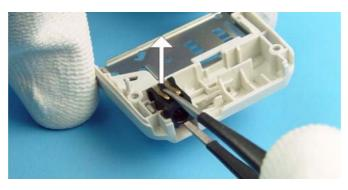
17. Use a flathead screwdriver as a lever to remove the release spring.
