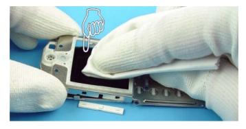
8. Always protect the LCD window with a protection foil to avoid dust and
