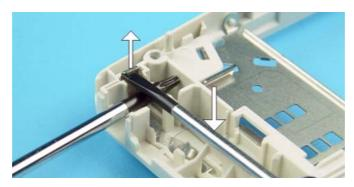
18. Turn the B-cover as shown to allow the release button to fall out.
