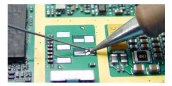
5. Place the connector between the markings and solder the first support angle. If
