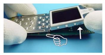
7. Separate the LCD from the UI shield by pressing out the LCD using a clean cloth. Prevent the key dome tape from getting dirty.
