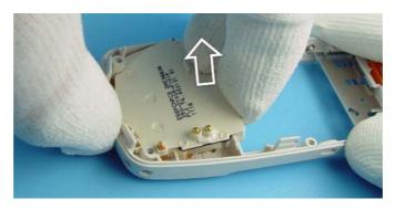
14. Use tweezers to remove the vibra motor.
