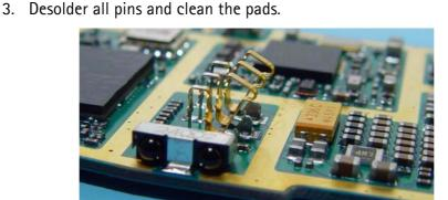
You need a soldering iron with a higher temperature when cleaning or soldering the ground pad.
