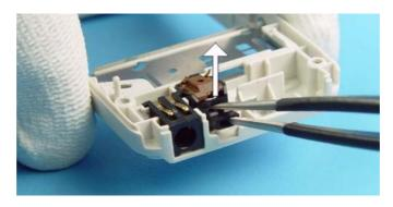
16. To remove the DC jack, place tweezers between the spring contacts and under
